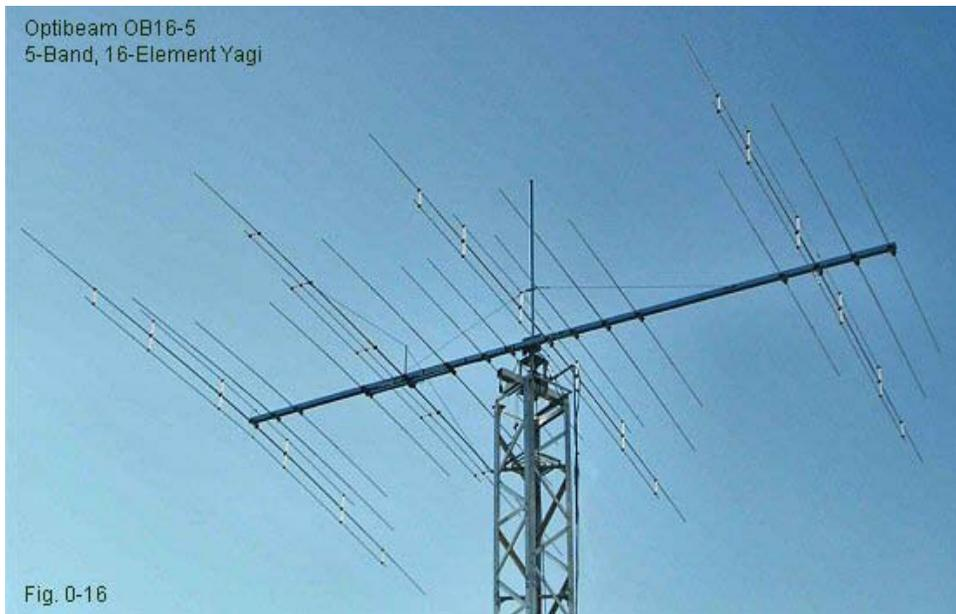
The sample is a photograph of an Optibeam OB16-5: a 5-band 16-element Yagi for the upper HF region. Although we count this as 16 elements linearly along the boom, note that several parasitic elements are multiples, with elements for three bands stacked vertically. However, before we can reach the level of designing a beam so complex, we must master a number of fundamentals.
