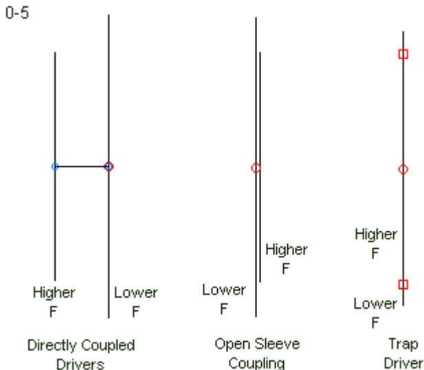
Three Common Types of Multi-Band Beam Feeding
