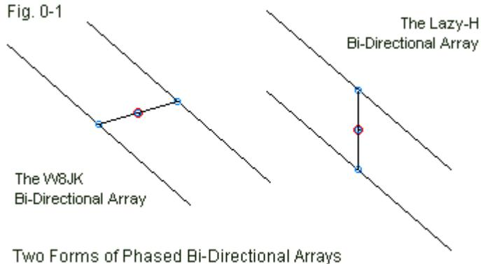
Both arrays use phase lines to establish the desired current magnitude and phase angle on each of the two elements. Phased arrays need not be bi-directional. **Fig. 0-2** shows the outline and an overlaid free-space E-plane pattern
