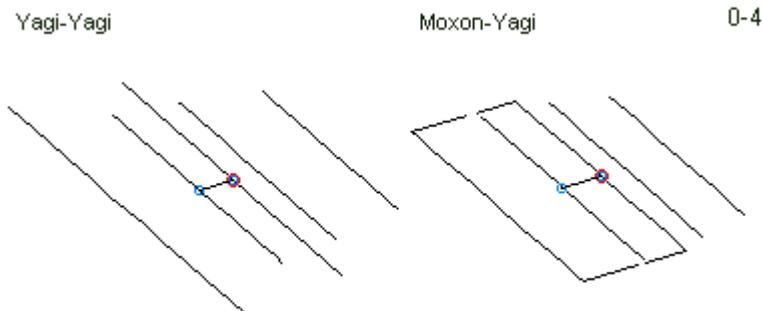
Outlines of Two Different 2-Band Parasitic Beams
