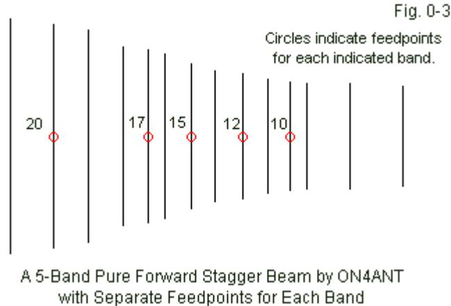
What rules out these beams from our work is the use of separate feedpoints for each section of the beam. When we think of a multi-band beam, we usually envision interlaced elements with a common feedpoint and a single feedline serving the entire array. We shall focus on these interlaced parasitic antennas.
