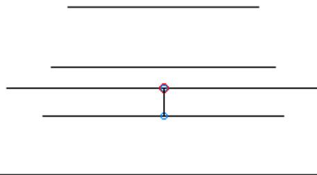
Replacing a Moxon Section with a Yagi Section
