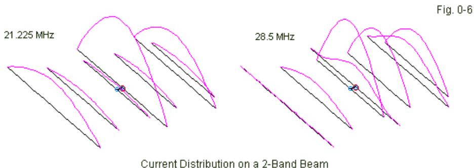
We shall also learn how to develop reasonable expectations from multi-band beams and to use—as sampled in **Fig. 0-6**—current distribution among array elements as an indicator of performance. In the course of these introductory notes, we shall also examine some of the modeling and construction challenges that go into these antennas.
