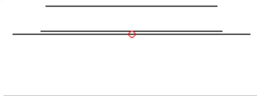
2-Band Yagi-Yagi: Sleeve Coupling
